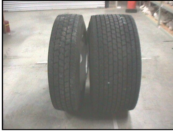
6 7 FIGURE 1. Wide-base single (445/50R22.5) and on tire of dual-tire assemblies 8 (275/80R22.5). 9
