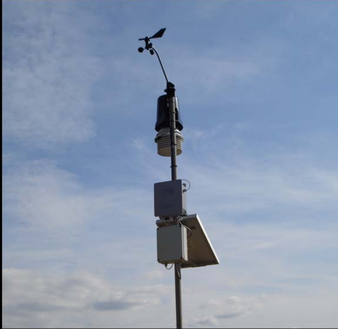
Typical setup of a Weather station
