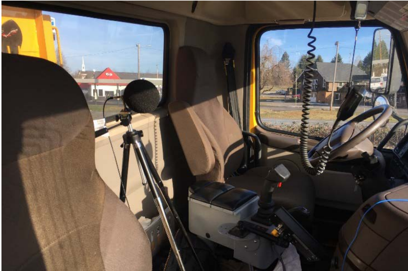
Heavy Vehicle Interior Microphone Setup
